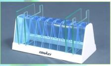
GENECO offers a complete range of Vertical Gel Units that combines the ease of use with high resolution separations. REGULAR as well as DUAL Models are available to run two gels simultaneously.
